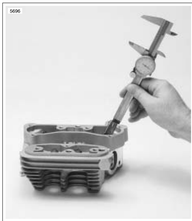
Figure 3-71. Measuring Valve Stem Protrusion
