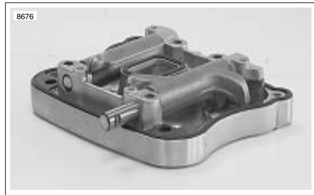
Figure 3-62. Removing Rocker Arm Shafts
