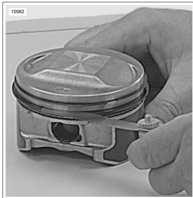
Figure 3-99. Measuring Ring Clearance in Groove
