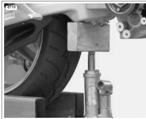
Figure 3-26. Supporting the Swingarm
