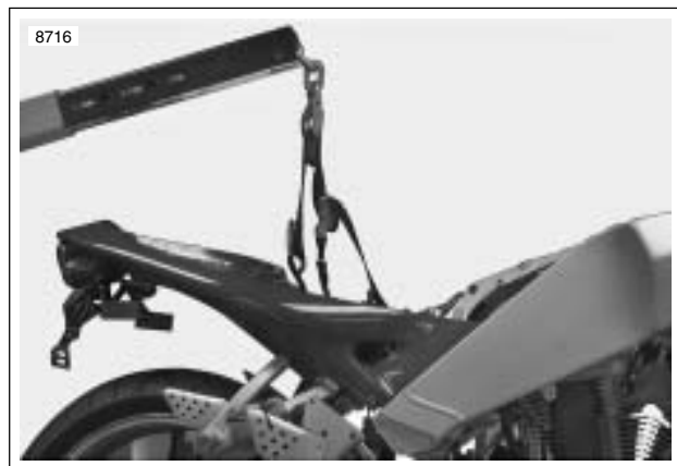
Figure 3-41. Supporting Vehicle for Assembly (Typical)
