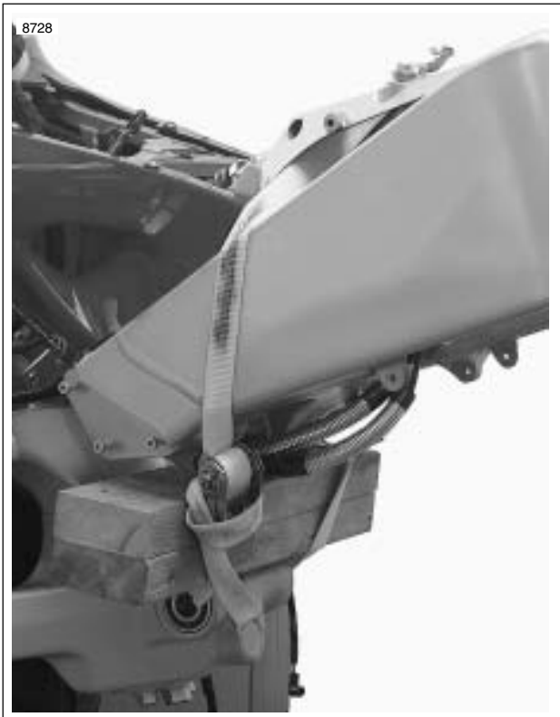
Figure 3-32. Securing Vehicle for Relocation (Typical)
