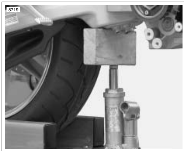
Figure 3-38. Supporting the Swingarm
