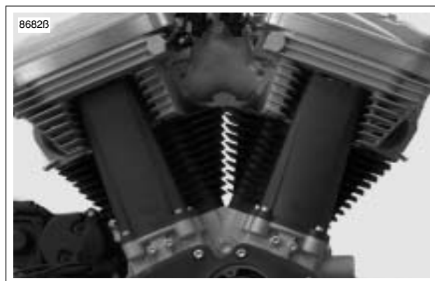
Figure 3-83. Push Rod Locations
