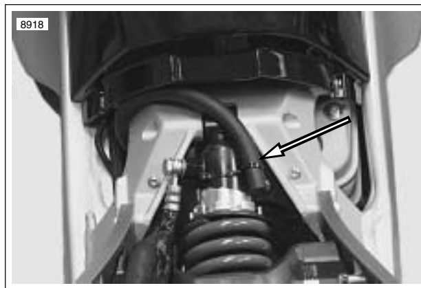
Figure 3-27. Transmission Vent Line
