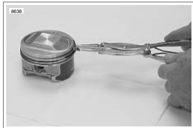
Figure 3-92. Removing Piston Rings
