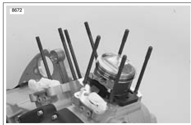
Figure 3-108. Piston Support Plate
