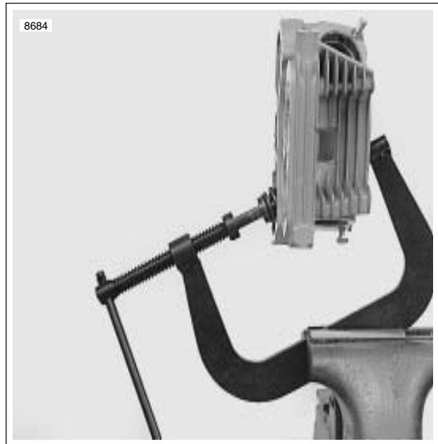
Figure 3-82. Valve Spring Compressor (Part No. HD-34736B)
