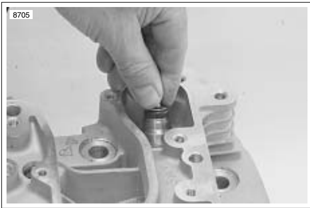
Figure 3-81. Valve Seal and Lower Collar Assembly Installation
