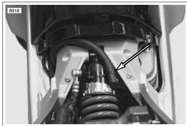
Figure 3-40. Transmission Vent Line
